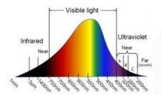
Most Safety Eyewear are inherently made from polycarbonate (PC) substrates which filter Ultraviolet Rays in the 200Nm to 400Nm range. But there are some operations that are performed which add an even higher level of danger when using certain types of equipment like curing or bonding lights. The light they emit requires additional protection using special lenses that protect up to 550Nm. Welding and Lasers may necessitate protection further in the Infrared (IR) range.
